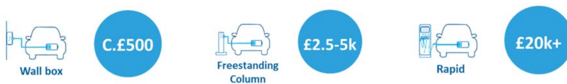
Figure 3. Typical installation costs (excluding chargers).
